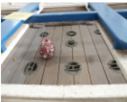
Portland Lifeboat - Wells Patent Lifeboat valves
