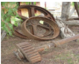
Remnant log winch mechanical parts - gears and counter shaft. March 2007.
