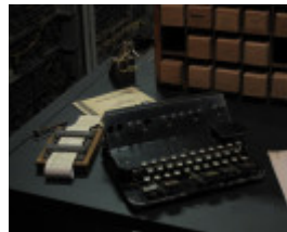
PROV H2217 CSIRAC close up of paper tape punch machine and tape holder
